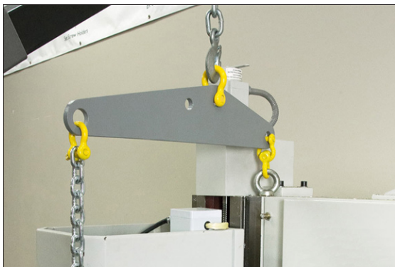
Figure 4-15: Lifting Bar Kit connected to the machine.
