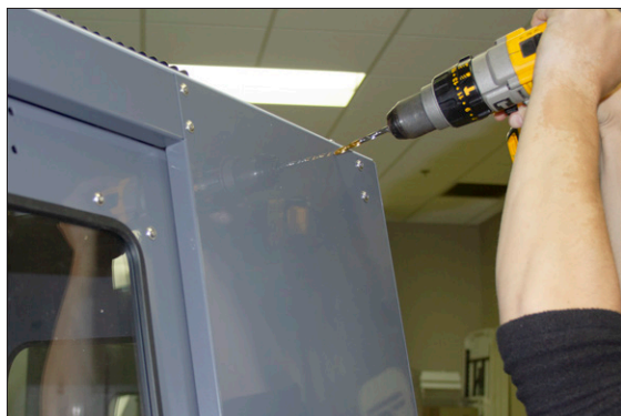
Figure 4-174: Drilling holes into the top of the enclosure.
