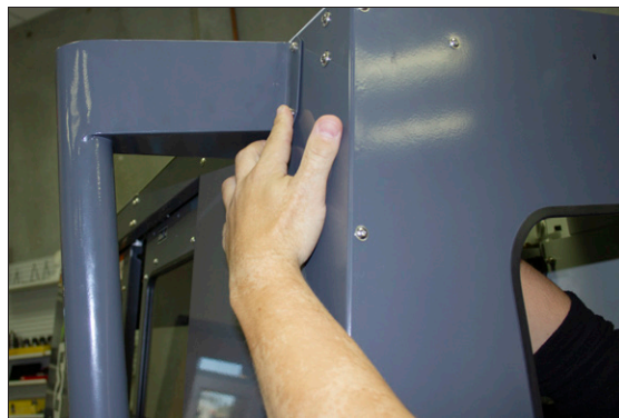
Figure 4-175: Securing the top of the mount arm to the enclosure.
