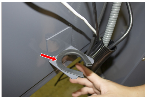
Figure 4-190: Rubber attached to the bracket on the keyboard tray.
