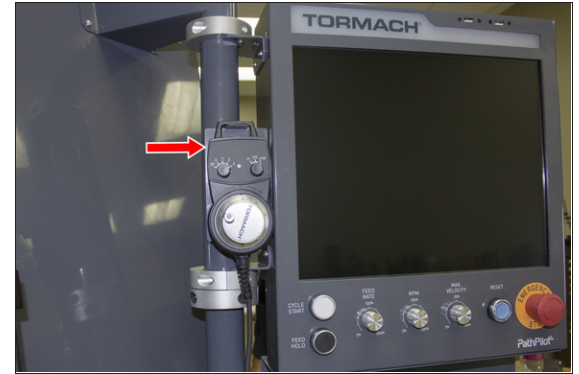
Figure 4-188: Jog pendant on the front of the console assembly.
