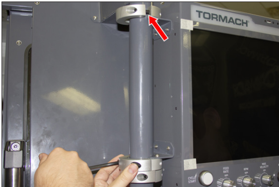
Figure 4-186: Loosely attaching the split collars to the mount arm.
