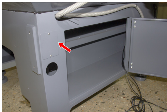
Figure 4-192: Access panel on the machine stand.
