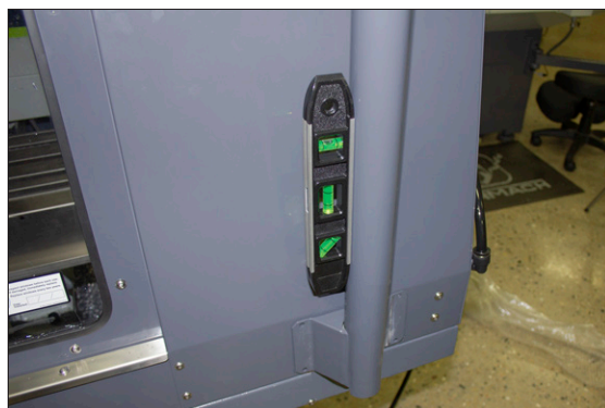
Figure 4-176: Bottom of the mount arm level on the enclosure.
