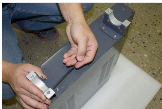
Figure 4-183: Split collars attached to the mount arm brackets on the controller.
