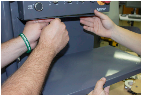
Figure 4-187: Attaching the keyboard tray to the bottom of the controller.
