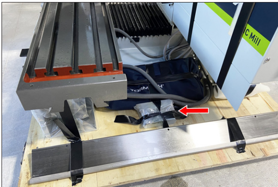
Figure 4-6: Y-axis bellows spacers on the pallet.
