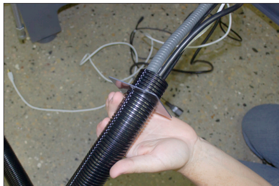
Figure 4-193: Loose end of corrugated tubing and all cords put through the access panel.
