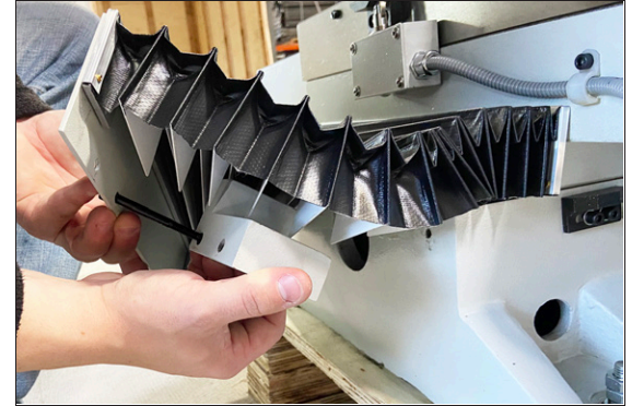
Figure 4-7: Installing the Y-axis bellows spacer.
