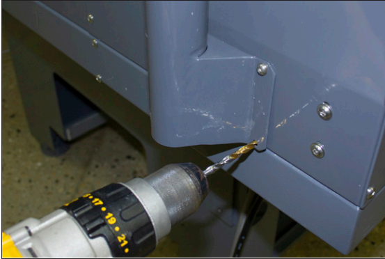
Figure 4-177: Drilling the remaining three holes into the enclosure.
