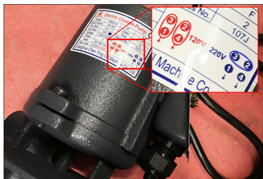
Figure 4-71: Coolant pump motor jumper configuration diagram.
