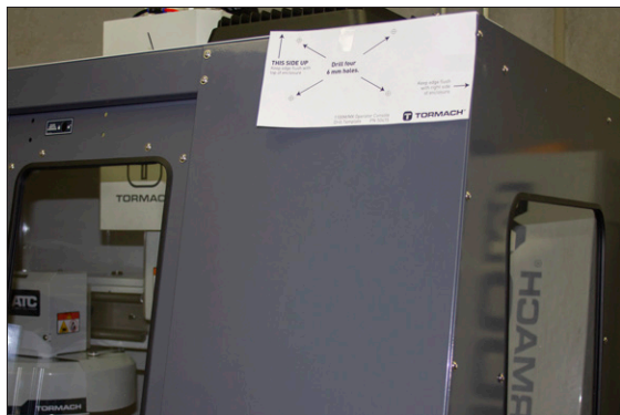
Figure 4-173: Drill template taped to the enclosure.
