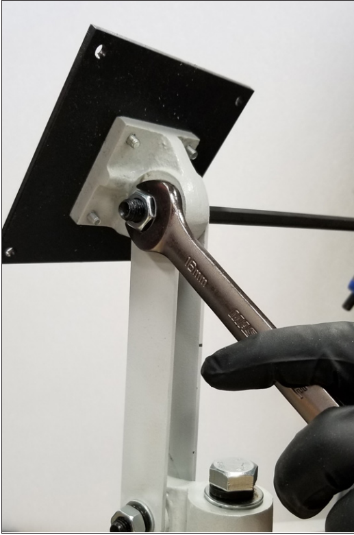
Figure 4-23: Tightening the monitor bracket in place.
