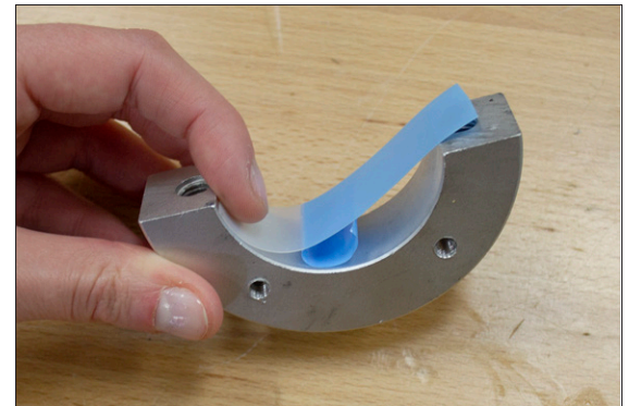
Figure 4-180: Adhering tape on the inside of a split collar.
