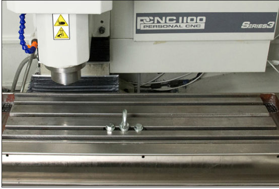
Figure 4-14: Lifting Bar Kit hardware arranged on the machine table.
