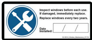
Figure 39: Window maintenance label.
