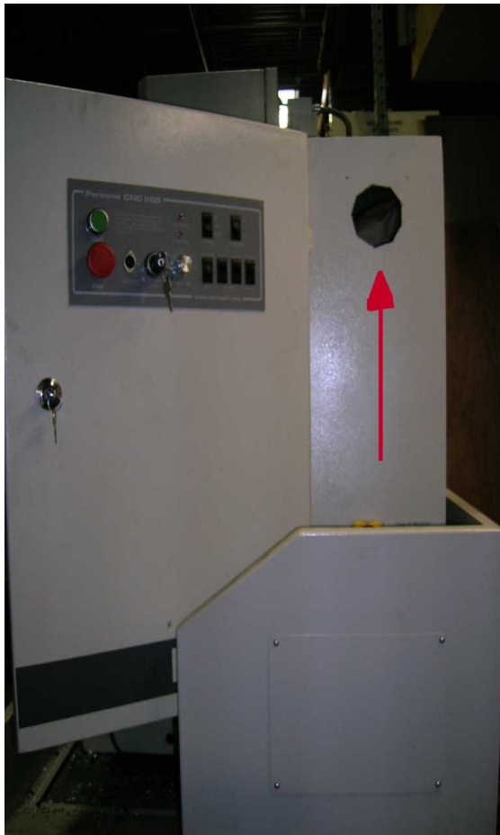
Upper vent cut out with die grinder
