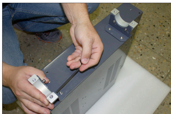
Figure 4-178: Split collars attached to the mount arm brackets on the controller.
