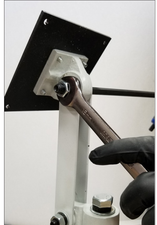
Figure 4-18: Tightening the monitor bracket in place.
