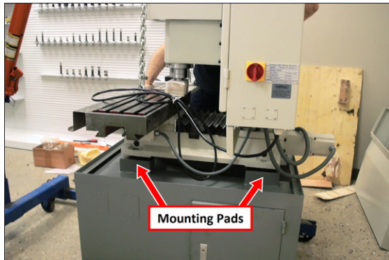
Figure 4-14: Machine lowered on to the mounting pads on the machine stand.
