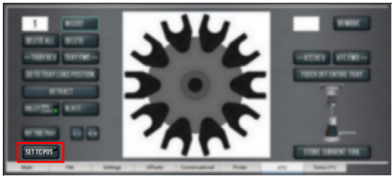
Figure 4-95: Set TC POS button on the ATC tab. The tool change position is set.
