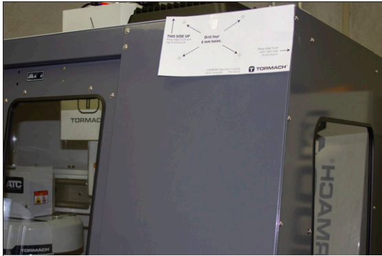
Figure 4-168: Drill template taped to the enclosure.
