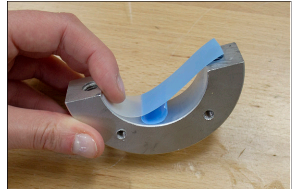
Figure 4-175: Adhering tape on the inside of a split collar.
