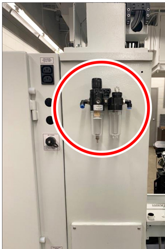
Figure 4-54: FRL installed on the machine.
