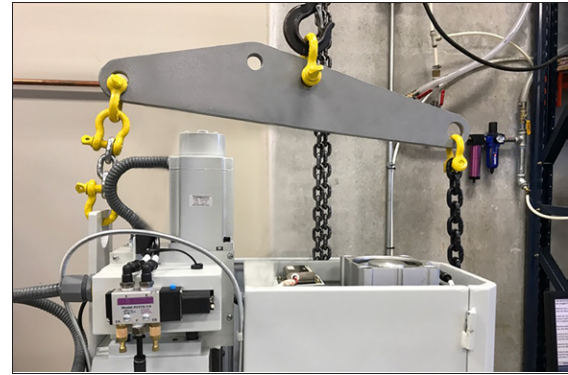
Figure 4-12: Lifting Bar Kit connected to the machine.
