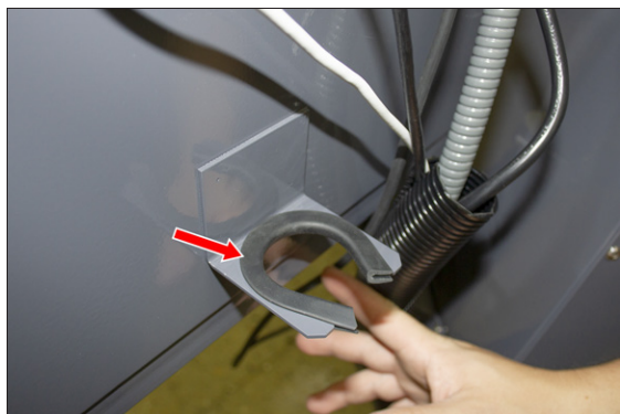
Figure 4-185: Rubber attached to the bracket on the keyboard tray.
