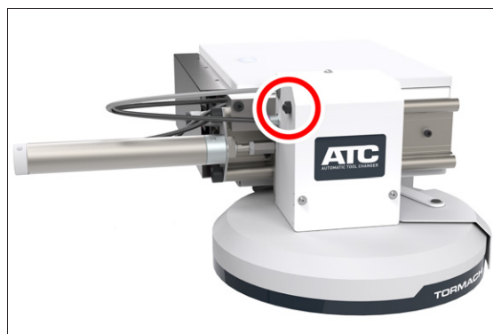
Figure 4-85: Collet open button on the side of the ATC.
