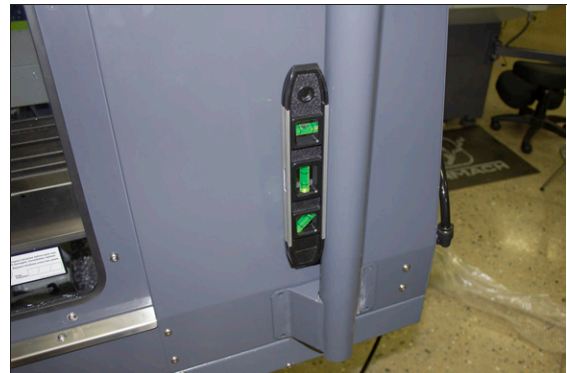
Figure 4-171: Bottom of the mount arm level on the enclosure.
