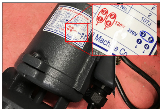
Figure 4-66: Coolant pump motor jumper configuration diagram.
