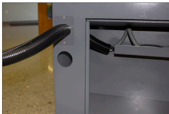
Figure 4-189: Access panel attached to the machine stand.
