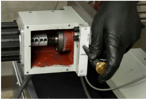
Figure 3: Center punch aligned on the front template.
