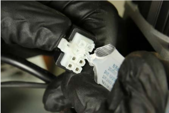
Figure 9: Dielectric grease on the Molex connector.
