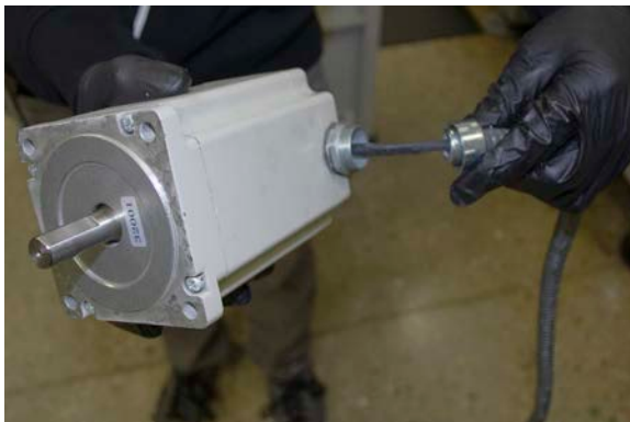
Figure 15: Removing the flex conduit from the X-axis motor.
