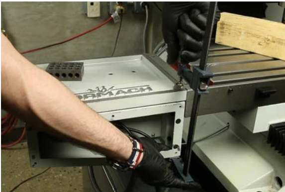
Figure 14: Clamping the tool tray to the X-axis motor cover.
