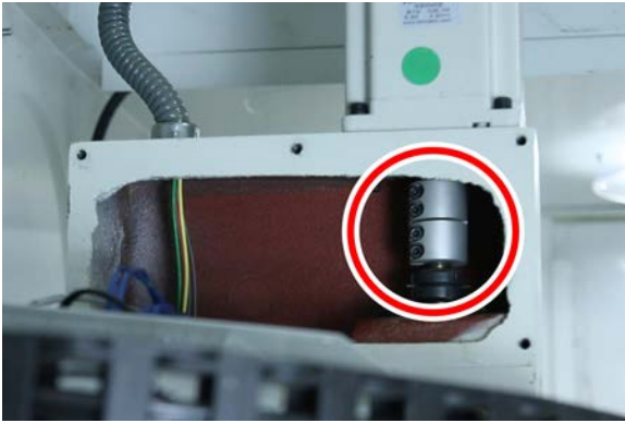
Figure 10: Set screws on the Z-axis coupler pointing toward the left side of the machine.
