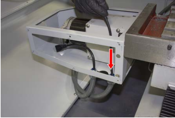
Figure 8: Routing the wires through the flex conduits.
