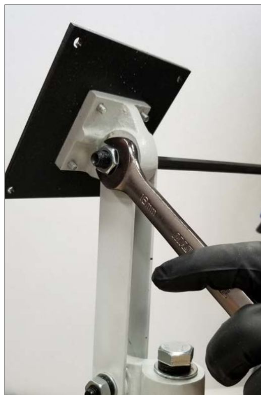
Figure 4-22: Tightening the monitor bracket in place.
