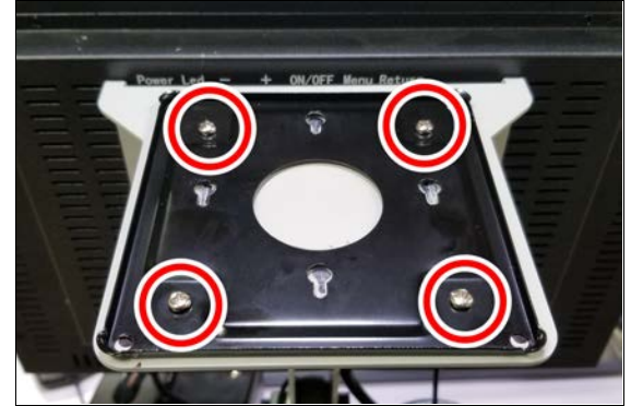
Figure 4-25: VESA plate mounted onto the PathPilot Controller VESA Mount (PN 50382).
