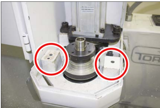
Figure 4-47: Mounting surfaces to clean inside the spindle motor cabinet.
