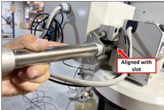
Figure 4-88: Installing the air cylinder into the ATC.
