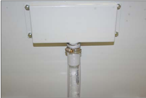
Figure 4-74: 3/4 in. ID clear tubing attached to the funnel tray.
