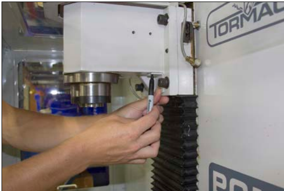
Figure 4-79: Relocation bracket used as a template to mark the hole locations.
