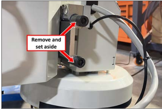
Figure 4-87: Bolts for the air cylinder pre-installed on the ends of the ATC's linear rail.
