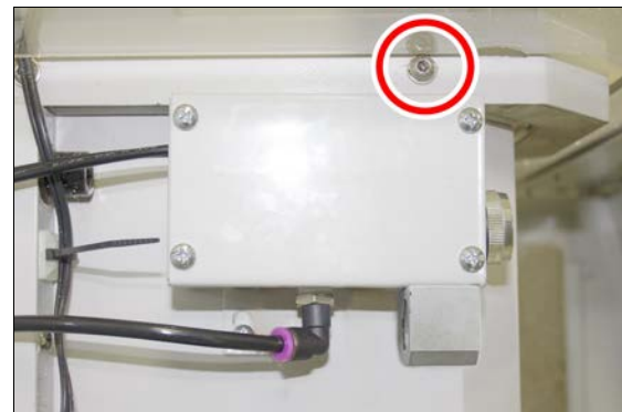
Figure 4-64: M6 × 12 mm socket head cap screw to remove.
