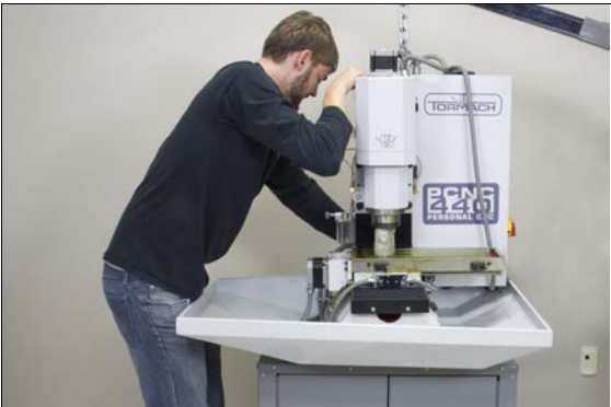
Figure 4-17: Lowering the machine onto the stand.
