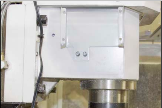
Figure 4-58: Button box base installed on the mill head.
