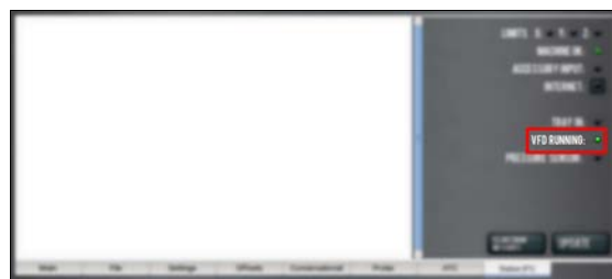
Figure 4-96: VFD Running light on the Status tab.
