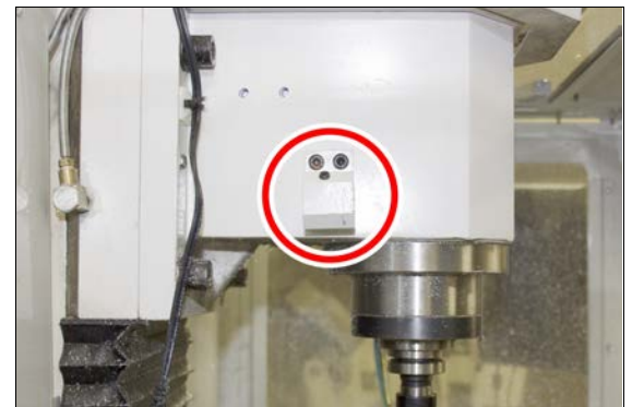
Figure 4-57: Coolant hose mount bracket on the mill head.
