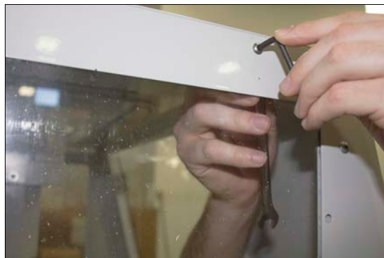
Figure 4-135: Example of securing a lock nut to a safety screw.
