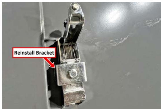
Figure 4-10: Attaching the door latch to the door with the bracket.
