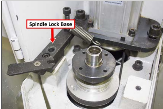
Figure 4-46: Spindle lock base from the original drawbar assembly.
