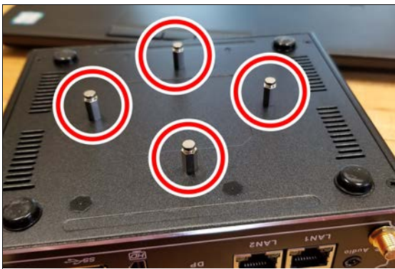
Figure 4-24: Installing the standoffs on the controller.
