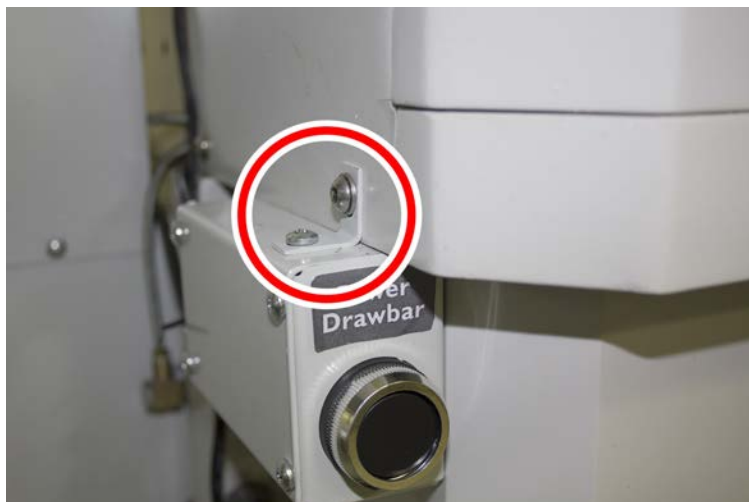
Figure 6: M6 \times 12 mm socket head cap screw on the Power Drawbar button assembly.
