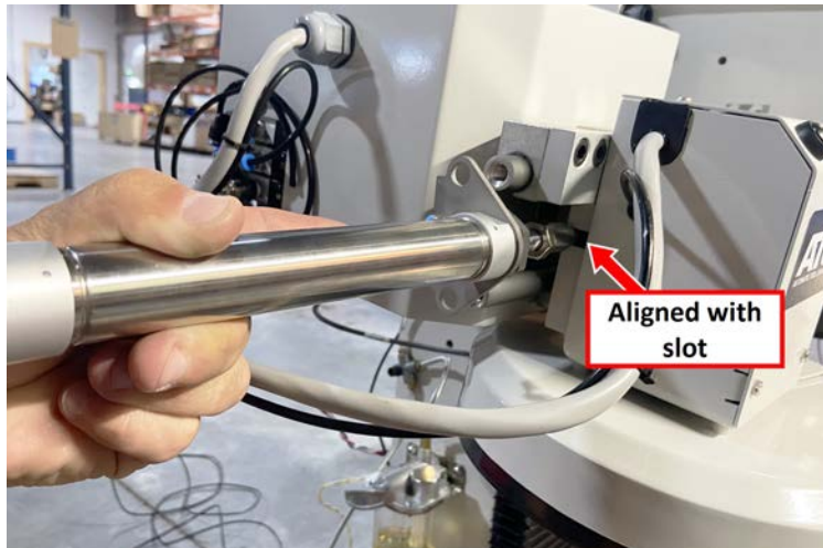
Figure 12: Installing the air cylinder into the ATC.
