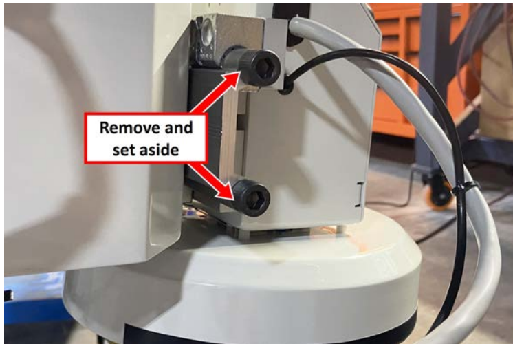
Figure 11: Bolts for the air cylinder pre-installed on the ends of the ATC's linear rail.
