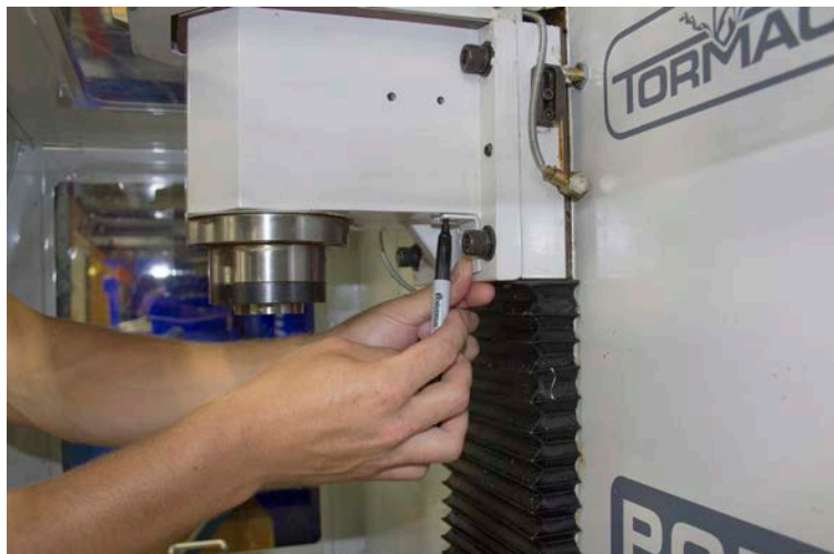
Figure 3: Relocation bracket used as a template to mark the hole locations.
