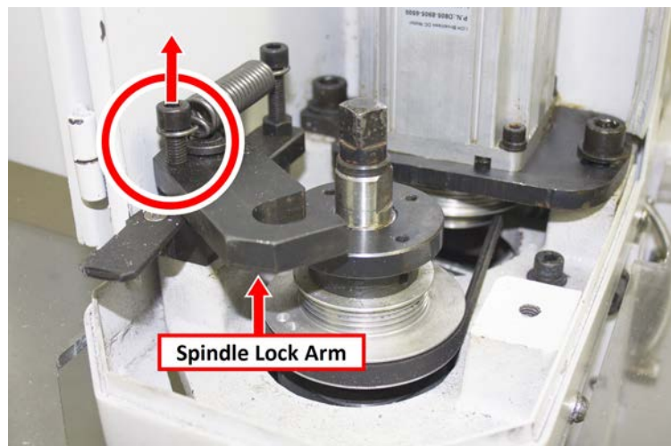
Figure 1: Spindle lock arm pivot screw removed from the original drawbar assembly.
