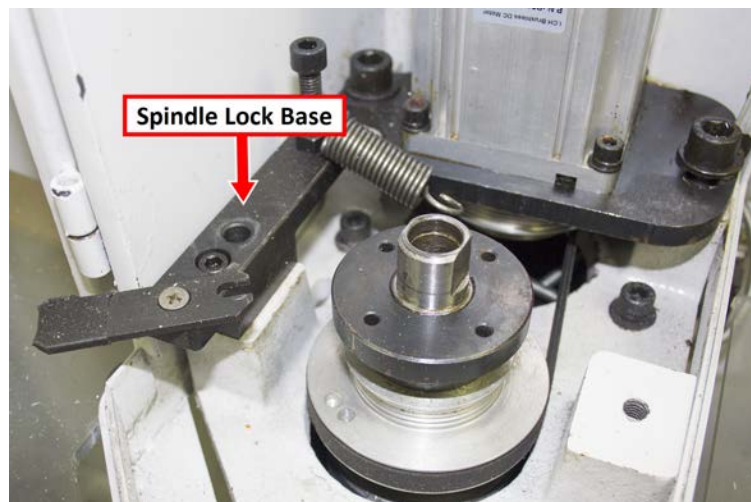
Figure 2: Spindle lock base from the original drawbar assembly.
