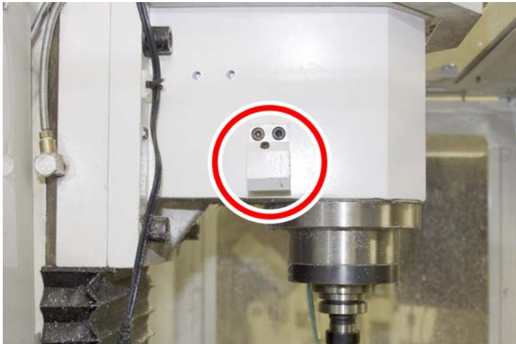
Figure 13: Coolant hose mount bracket on the mill head.
