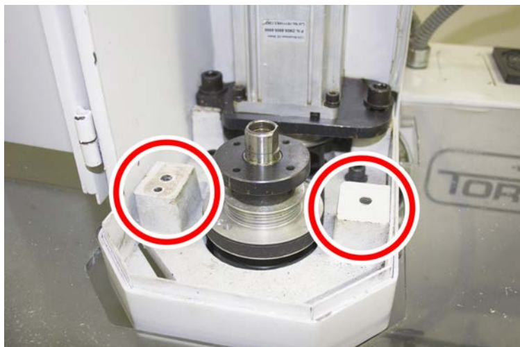
Figure 3: Mounting surfaces to clean inside the spindle motor cabinet.
