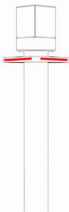
Figure 4: Convex side of the spring washer toward the drawbar head.
