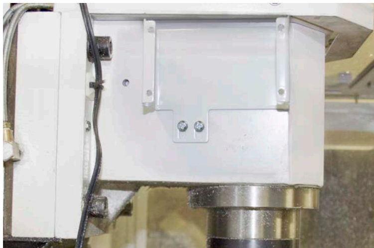
Figure 14: Button box base installed on the mill head.
