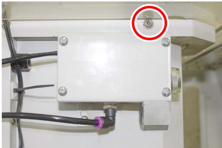
Figure 20: M6 × 12 mm socket head cap screw to remove.
