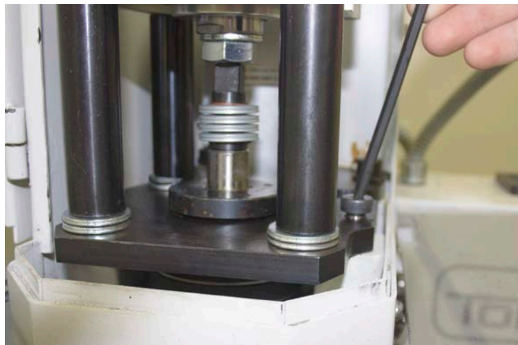
Figure 11: M10 × 16 mm shoulder screw installed on the Power Drawbar cylinder's mount plate.
