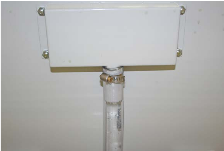
Figure 5: 3/4 in. ID clear tubing attached to the funnel tray.
