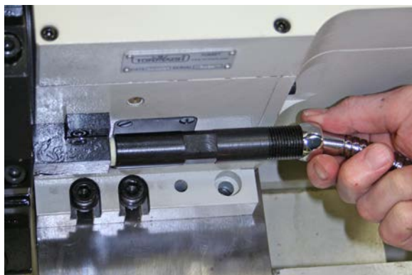
Figure 29: Installing the coolant hose onto the coolant fitting.
