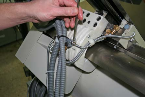
Figure 45: Disconnecting the oil line.
