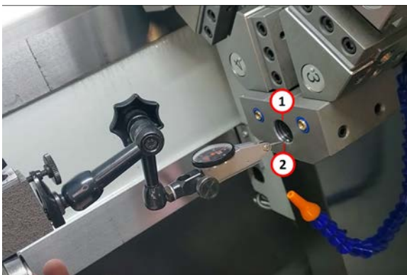
Figure 22: Positions to read the indicator.
