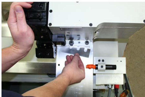
Figure 27: Installing a shim under the rear of the turret.
