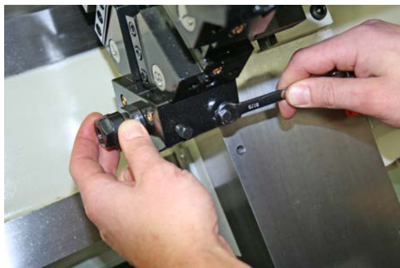
Figure 31: Installing a tool into the boring bar.
