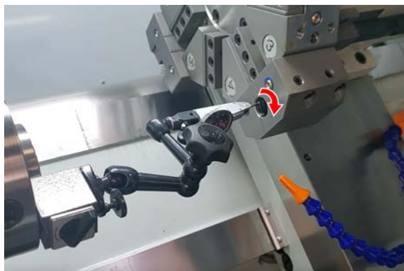
Figure 21: Indicator positioned within the boring bar holder.
