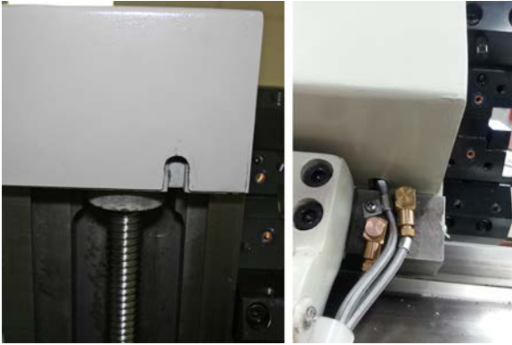
Figure 50: Oil line clearance checks.
