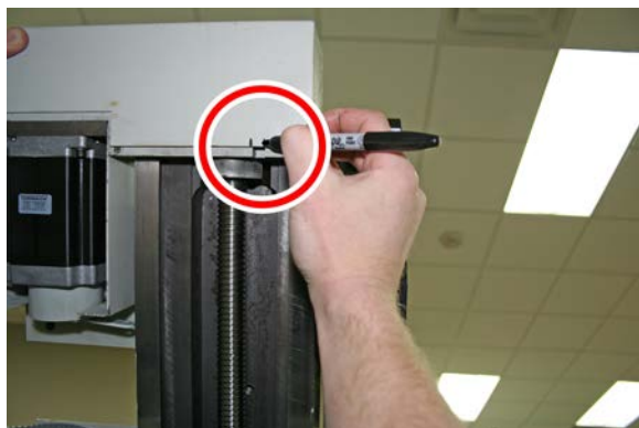
Figure 47: Marking the cutout location.
