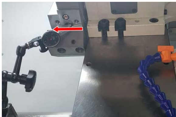
Figure 28: Sweeping the dial indicator across the Z-axis of the turret face.
