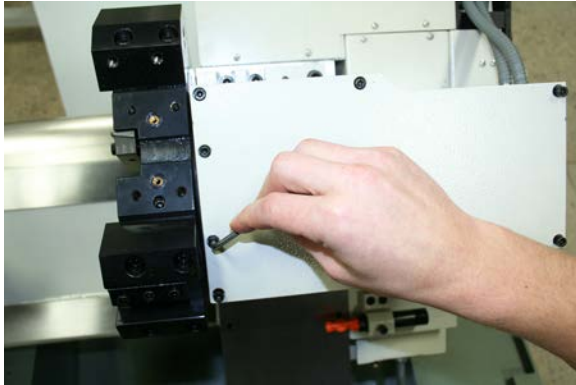
Figure 39: Removing the motor cover.
