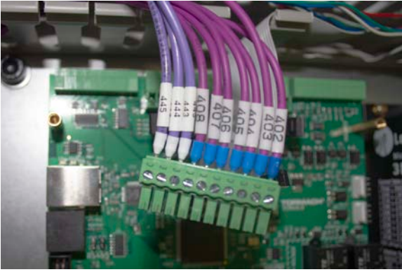
Figure 9: Final wire configuration for connector J1.
