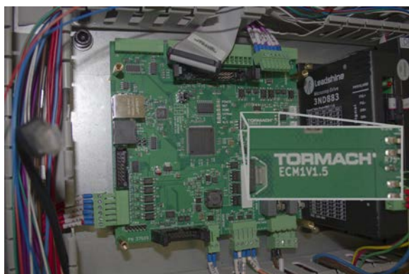
Figure 5: ECM v1.5 board installed in the electrical cabinet.
