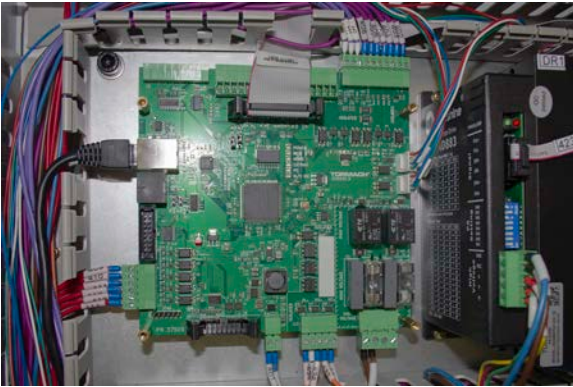
Figure 10: ECM v1.5 board correctly installed in the electrical cabinet.
