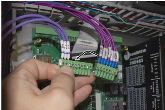
Figure 8: Wires from the old connector J1 and wires from the new connector J1.
