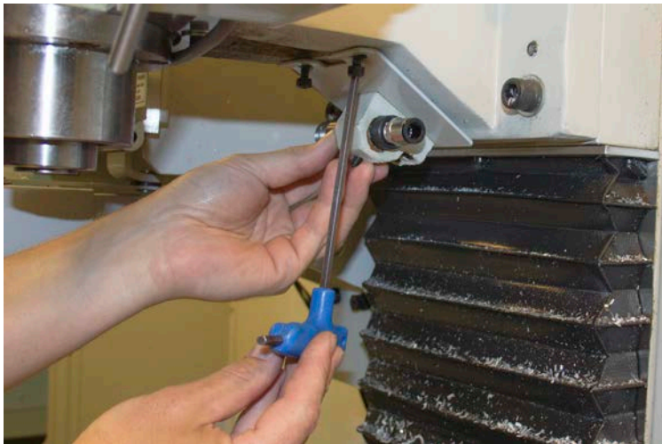
Figure 3: Relocation bracket mounted below the spindle head.
