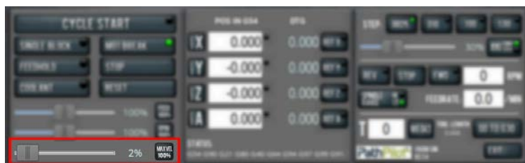
Figure 43: Maxvel Override slider on the Main tab.
