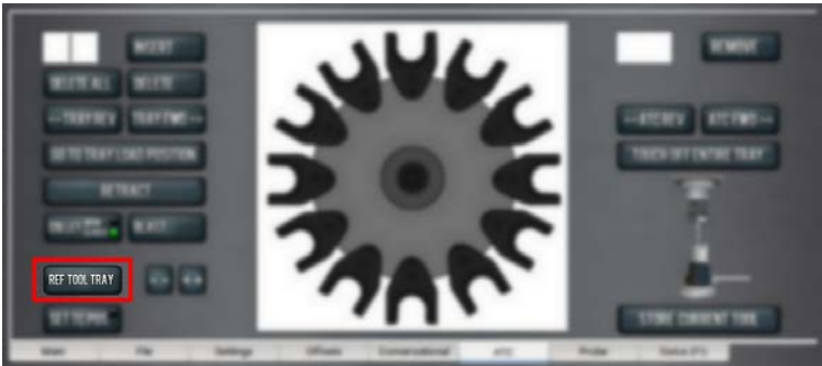
Figure 37: Ref Tool Tray button on the ATC tab.
