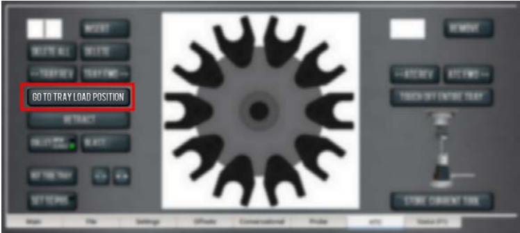
Figure 38: Go to Tray Load Position button on the ATC tab.
