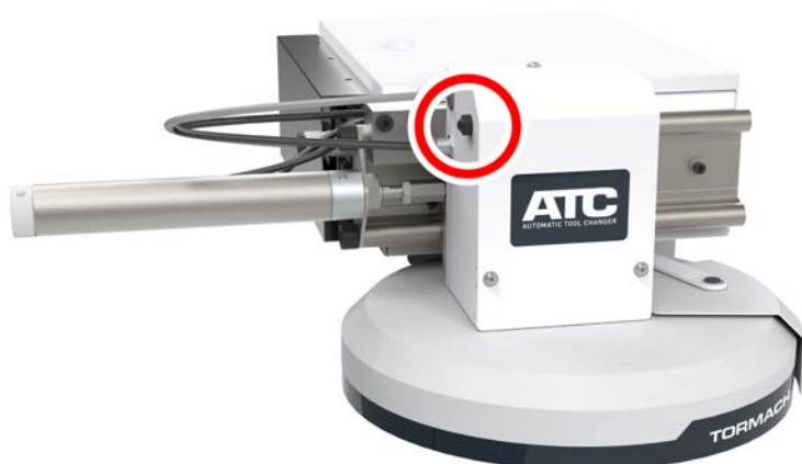
Figure 31: Collet open button on the side of the ATC.
