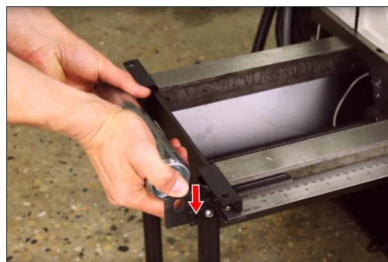
Figure 4-9: Squeezing the spring-loaded post.
