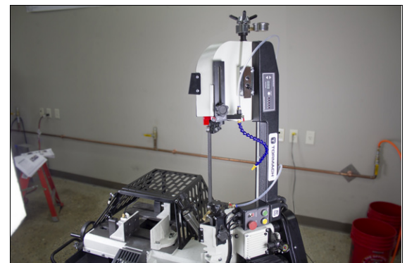
Figure 10-5: Bandsaw head lifted upright.
