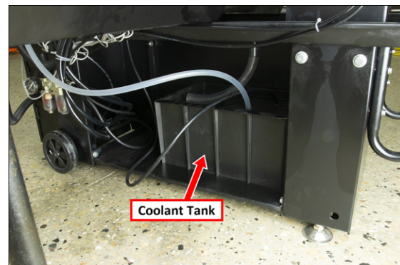
Figure 4-3: Coolant tank inside the machine's stand.
