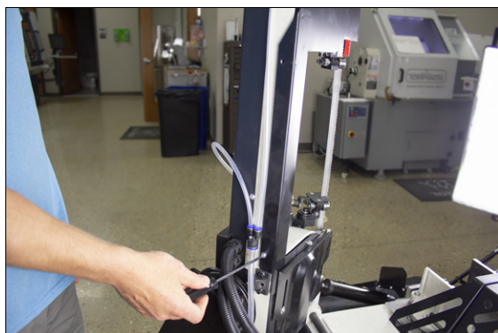
Figure 6-6: Removing the screws securing the blade cover to the bandsaw.
