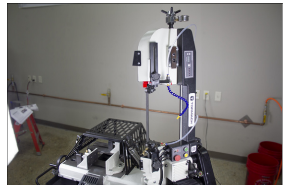
Figure 6-4: Bandsaw head lifted upright.
