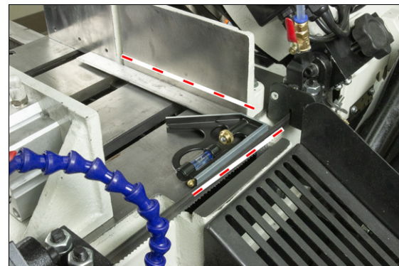
Figure 4-11: Fixed jaw aligned with the blade.
