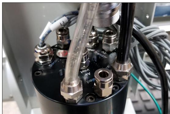
Figure 4-51: Water line connections.
