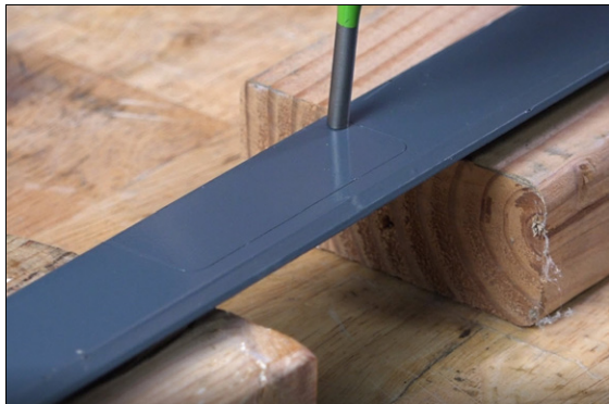
Figure 4-82: Using a punch to break the tab closest to the edge of the linear rail cover.
