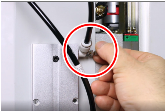
Figure 4-88: Loosening the dust shoe lift speed control valve.
