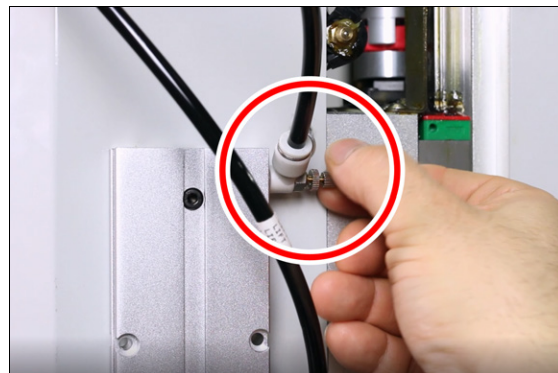
Figure 4-93: Loosening the dust shoe lift speed control valve.
