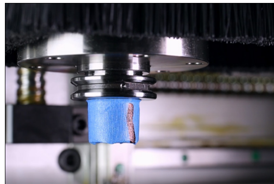
Figure 4-94: Tape and line indicator installed into the spindle.
