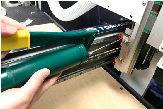
Figure 10-5: Lubricating a bearing block with the Grease Gun.
