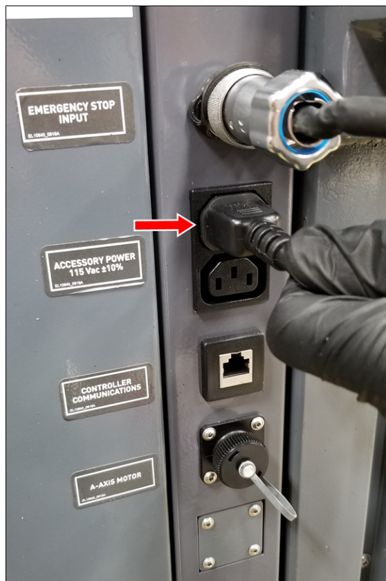
Figure 4-23: Connecting the monitor cable to the Accessory Power Port.
