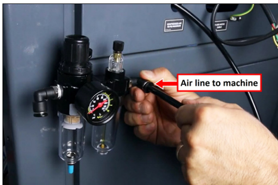
Figure 4-67: Connecting the machine's air line to the FRL.
