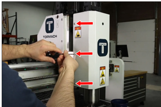
Figure 4-43: Removing the M5 screws that secure the front spindle cover.
