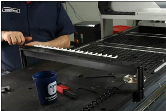
Figure 4-86: Installing the rack onto the standoffs.
