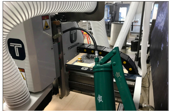
Figure 10-6: Lubricating a remote-mounted lubrication port with the Grease Gun.
