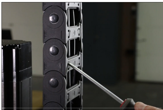
Figure 4-53: Removing pieces of the energy chain.
