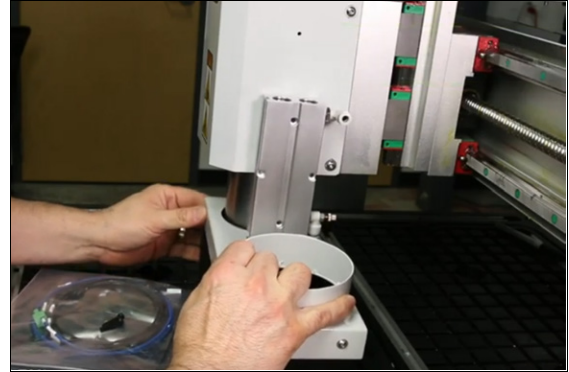
Figure 4-72: Sliding the dust shoe onto the spindle.
