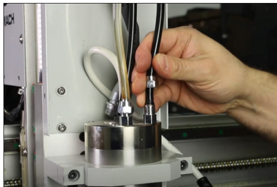
Figure 4-45: Two water lines on the existing spindle.
