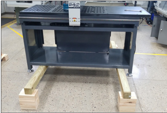
Figure 4-4: Pallet removed from the machine, which is now completely held by the boards.
