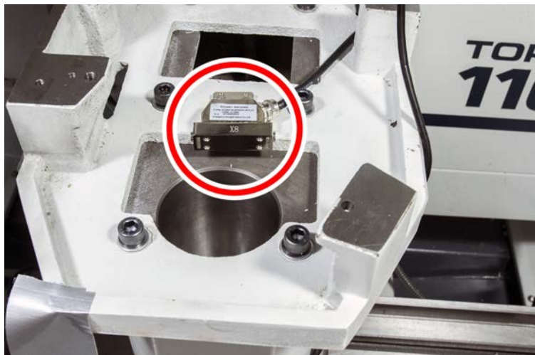
Figure 16: Encoder read head installed on the head casting.
