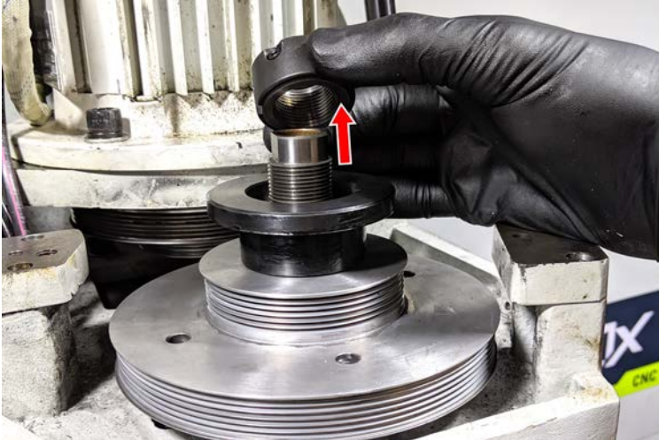
Figure 12: Removing the retention nut.
