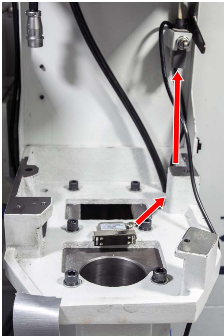
Figure 17: Encoder wiring management.
