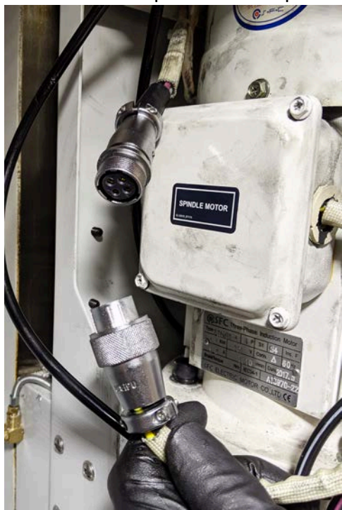
Figure 1: Spindle motor quick-connect fitting disconnected.
