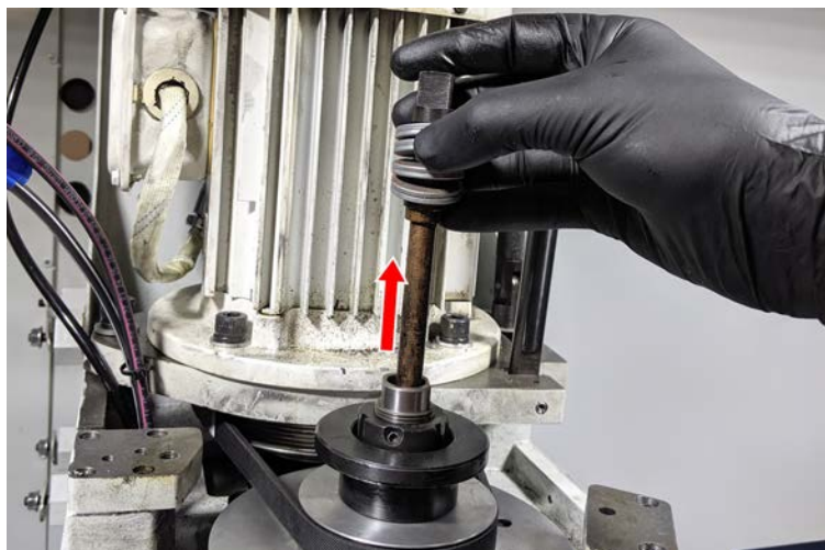
Figure 9: Removing the existing drawbar.
