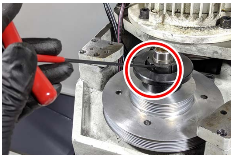
Figure 11: Loosening the retention nut's set screws.
