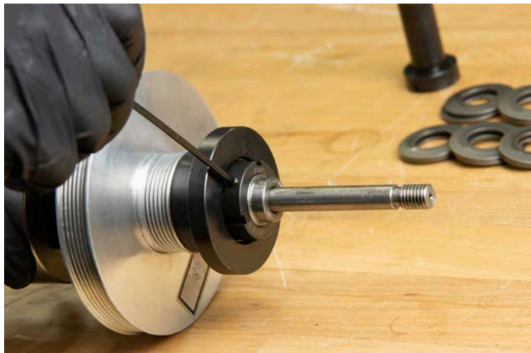
Figure 21: Preventing the drawbar shaft from rotating.
