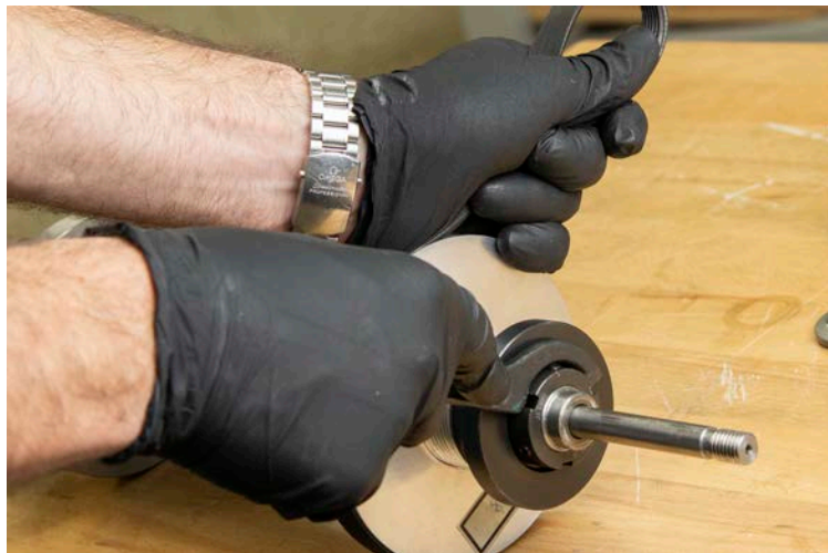
Figure 25: Removing the retention nut.
