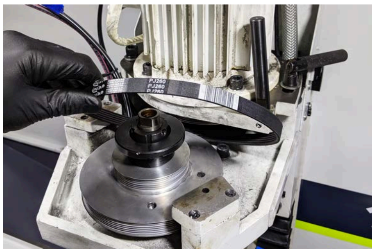
Figure 10: Removing the spindle belt.
