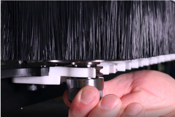
Figure 58: Rotating the tool holder to feel when the drag increases.
