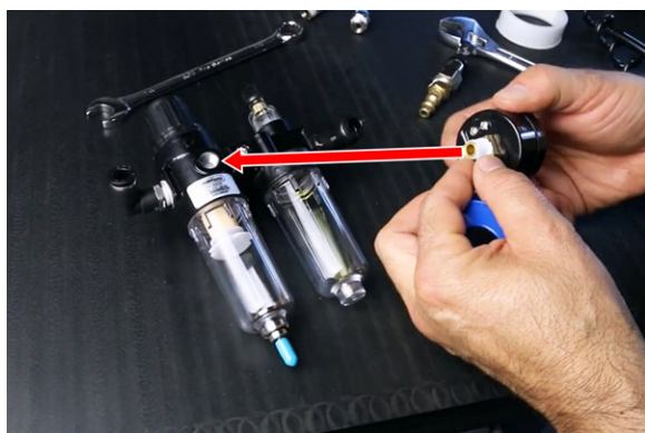
Figure 24: Preparing the dial for installation on the FRL.
