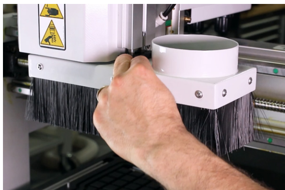
Figure 51: Pressing down on the dust shoe.
