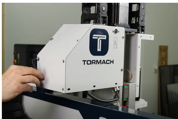
Figure 13: Rear Z-axis access panel.
