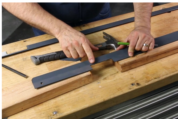
Figure 42: Linear rail cover with punch-out removed.
