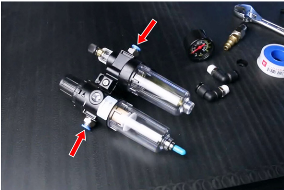
Figure 22: Preinstalled push-to-connect fittings on the FRL.
