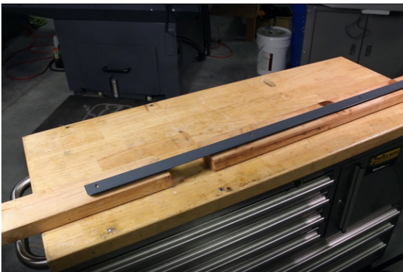
Figure 40: Linear rail cover on two wooden blocks.
