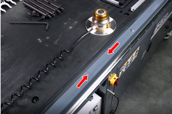
Figure 39: Linear rail cover punch-outs.
