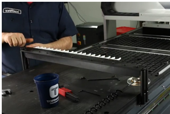
Figure 45: Installing the rack onto the standoffs.
