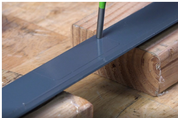
Figure 41: Using a punch to break the tab closest to the edge of the linear rail cover.
