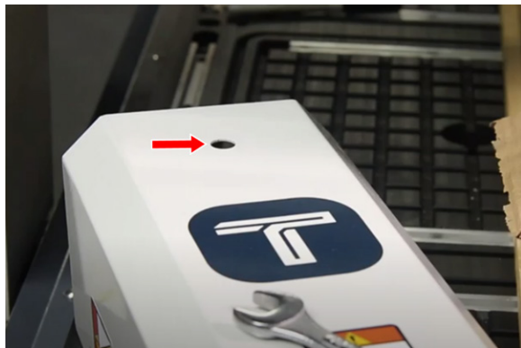
Figure 29: Power drawbar button hole on the spindle cover.
