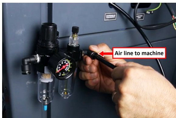
Figure 26: Connecting the machine's air line to the FRL.
