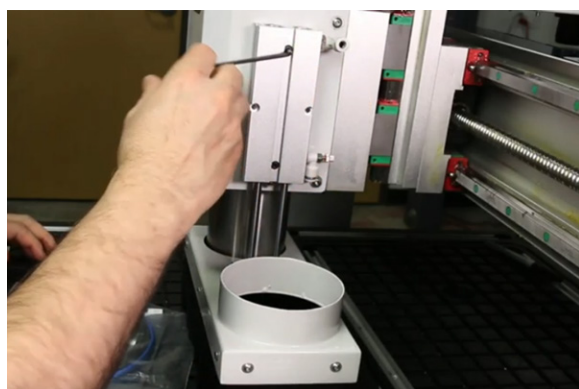
Figure 32: Mounting the dust shoe onto the spindle cover.
