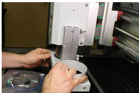
Figure 31: Sliding the dust shoe onto the spindle.
