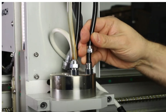
Figure 4: Two water lines on the existing spindle.
