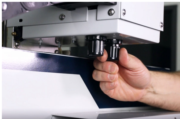
Figure 48: Unlocking the dust shoe extend pressure regulator.
