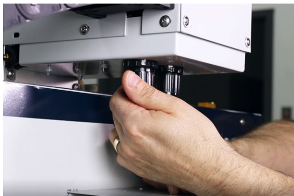
Figure 50: Unlocking the dust shoe lift pressure regulator.
