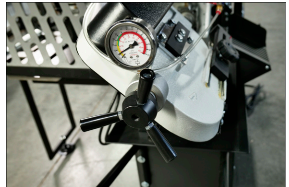
Figure 6-10: Tensioner dial aligned with the tip of the arrow.
