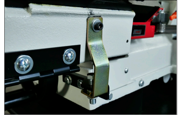
Figure 4-5: Shipping bracket securing the base casting to the head casting.
