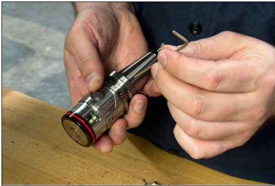
Figure 4-279: Installing the probe into the BT30 holder.
