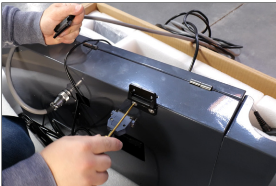
Figure 4-46: Installing the hinges onto the operator console.
