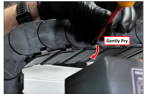
Figure 4-142: Removing the covers from the energy chain.
