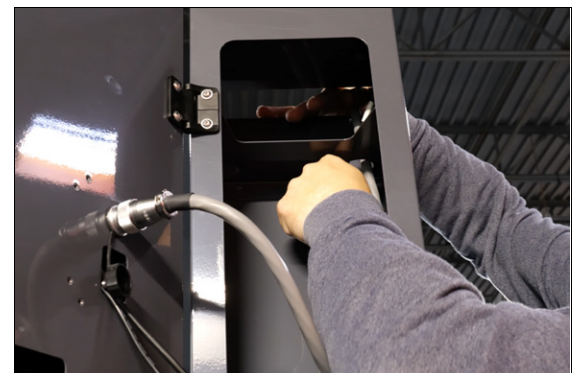
Figure 4-48: Routing the cables through the top operator console mount and to the top of the enclosure.
