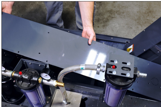
Figure 4-160: Installing the wide panel.
