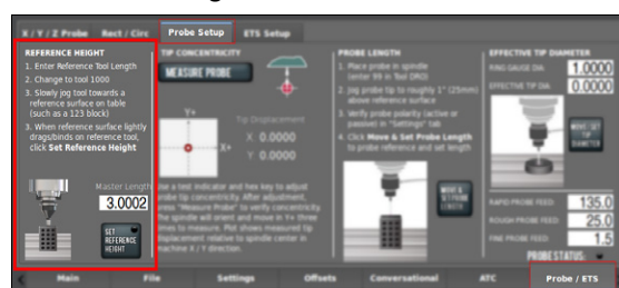
Figure 4-287: Reference height section of the probe setup.
