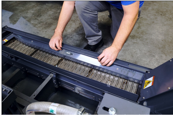
Figure 4-158: Installing the narrow panel.
