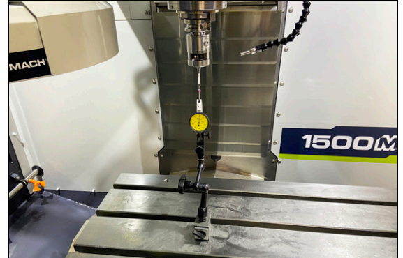
Figure 4-282: Dial indicator set up to check the probe's tip concentricity.
