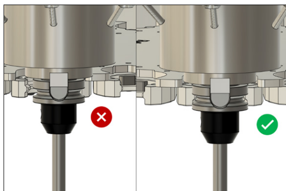
Figure 4-235: Examples of tool holder alignment vertically within the tool slots.
