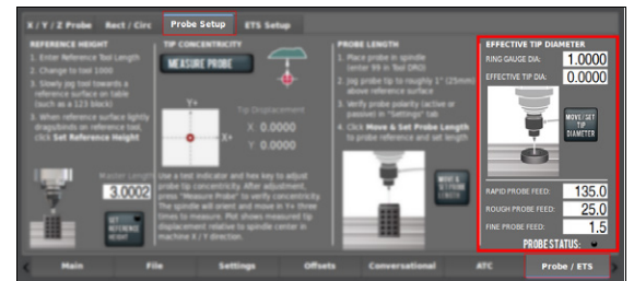
Figure 4-292: Effective tip diameter section of the probe setup.
