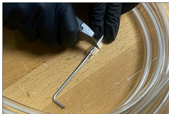
Figure 4-181: Cut the 3/8 in. tube away from the 1/8 in. capillary tube.
