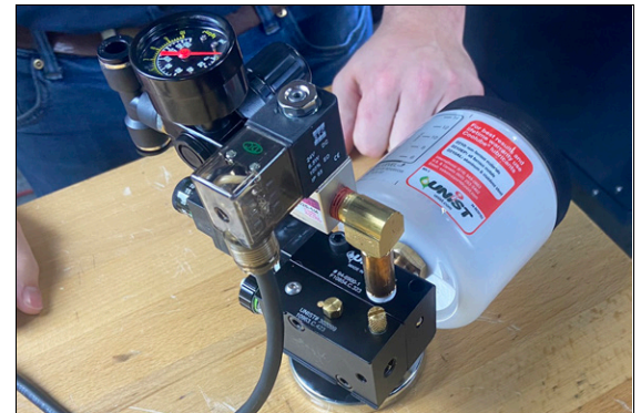
Figure 4-186: Solenoid mounted onto the coolant pump.
