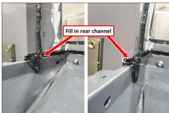
Figure 4-25: Example of sealant in the rear channel where the chip tray and machine casting meet.
