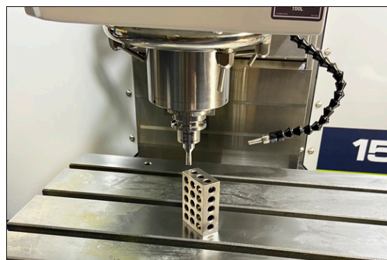
Figure 4-286: Calibration tool near the top of the 1-2-3 block.
