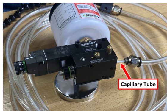
Figure 4-178: Push-to-connect fitting removed from the pump.
