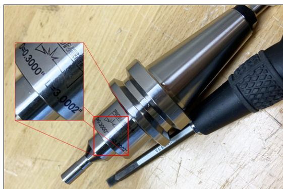
Figure 4-284: Diameter and length measurements engraved on to the calibration tool.
