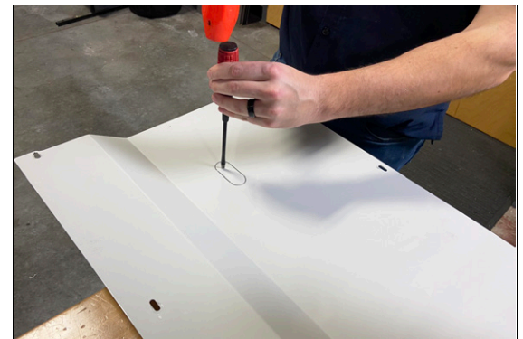
Figure 4-103: Knock-out hole on the right side spindle cover.
