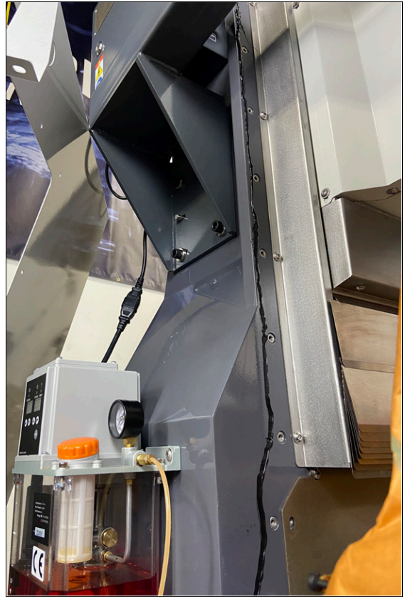
Figure 4-23: Example of sealant applied to the side of the machine column casting.
