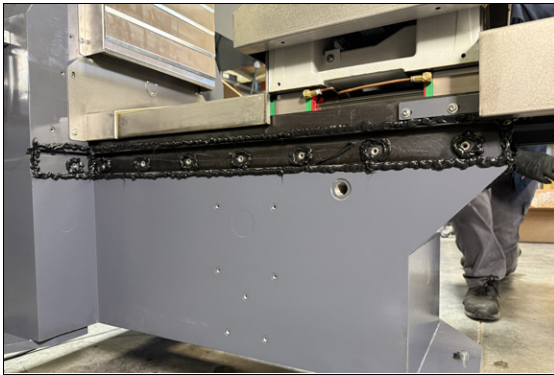
Figure 4-19: Example sealant application on the base of the machine.
