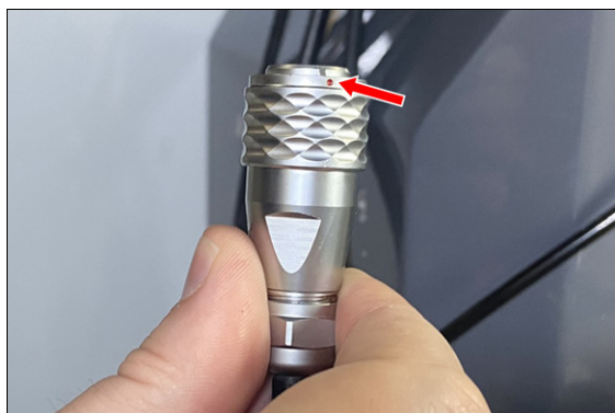
Figure 4-268: Red dot on the cable to align with the red dot on the connector.
