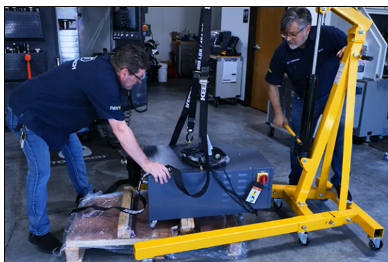
Figure 4-130: Removing the TSC pump from the pallet.
