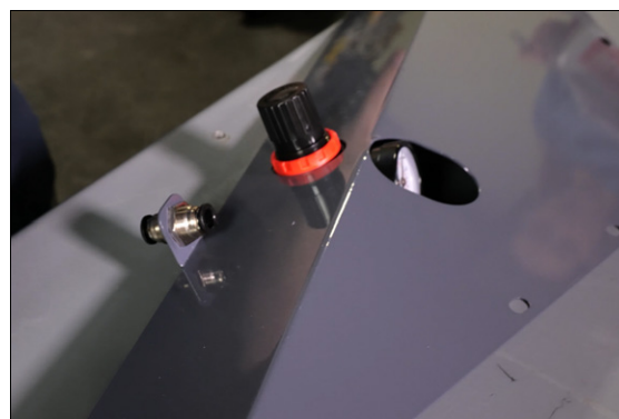
Figure 4-11: Bulkhead fitting and pressure regulator installed.
