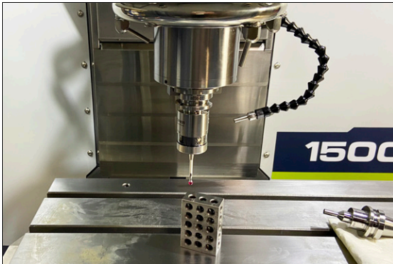
Figure 4-288: Probe tip near the top of the 1-2-3 block.
