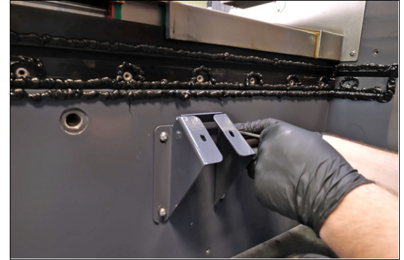
Figure 4-20: Installing a chip tray support bracket onto the machine stand.
