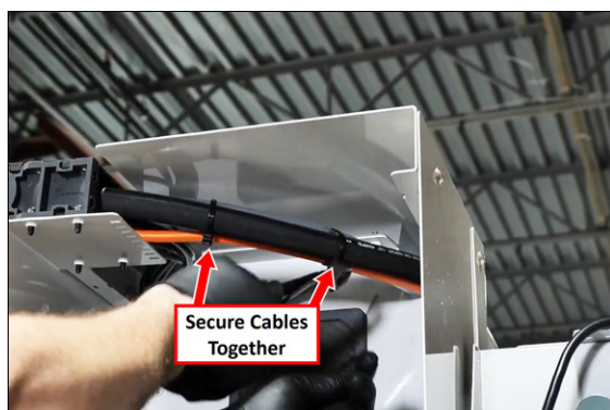
Figure 4-145: Securing the energy chain cables together.
