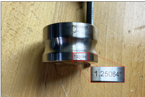
Figure 4-290: Diameter measurement engraved onto the ring gauge.
