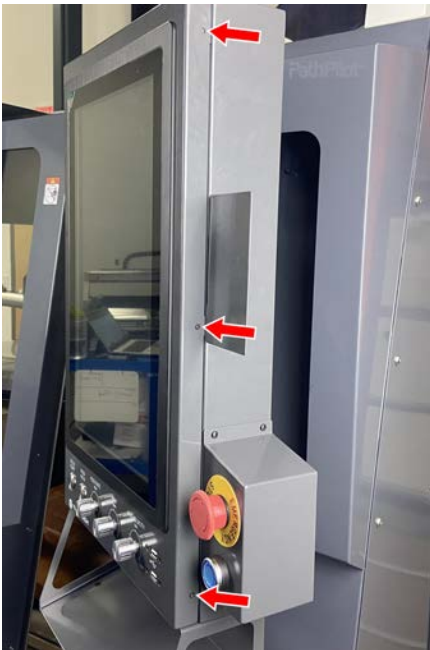
Figure 1: Screws securing the operator console's front panel.
