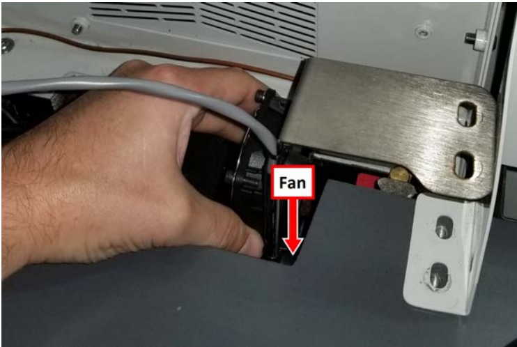
Figure 2: Lowering the fan into the space between the motor and the column.
