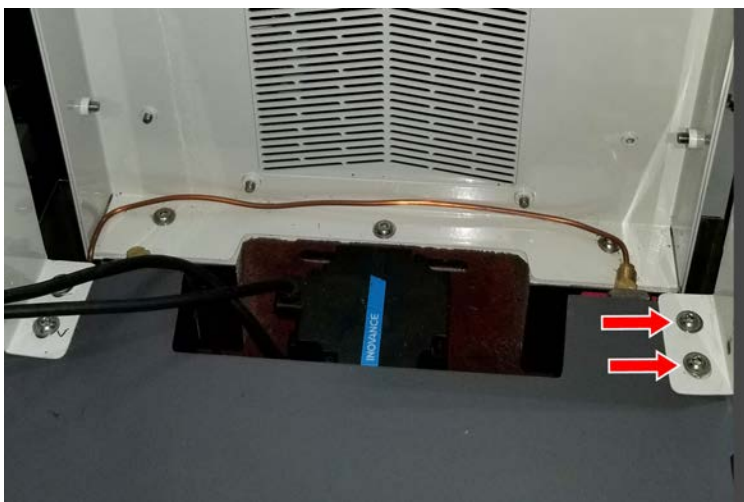
Figure 1: Screws attaching the enclosure to the column casting.
