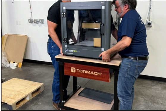
Figure 3-5: Lifting and placing the machine on the table.
