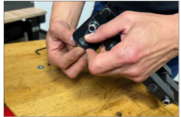
Figure 3-7: Installing the hardware onto the controller arm.
