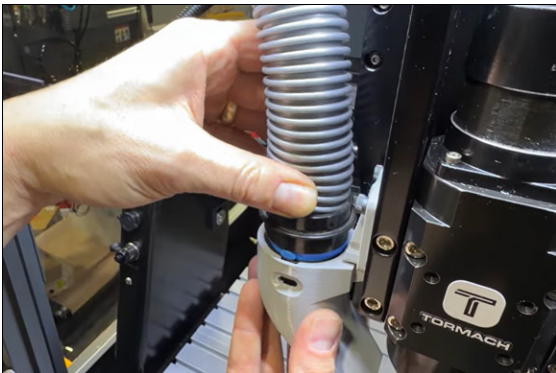
Figure 3-32: Connecting the hose to the dust boot.
