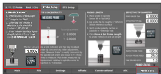
Figure 3-39: Reference height section of the probe setup.
