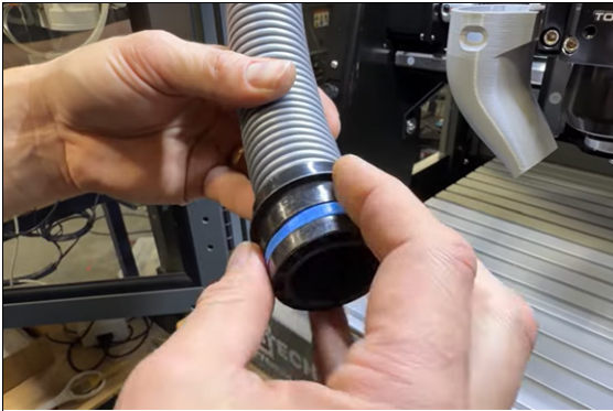
Figure 3-31: Threading the quick-connect piece onto the hose.
