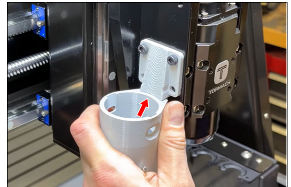
Figure 3-29: Pressing the dust boot into the bracket.
