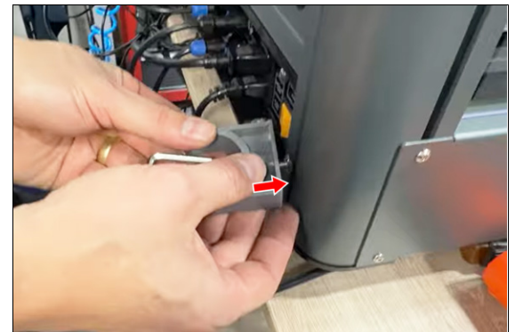
Figure 3-30: Sliding the hose bracket into the slot on the back of the machine.
