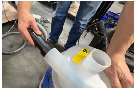
Figure 3-34: Attaching the hose to the dust separator.
