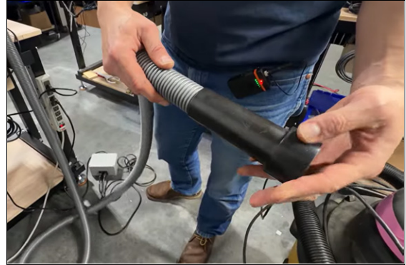
Figure 3-33: Threading the inlet connector onto the hose.
