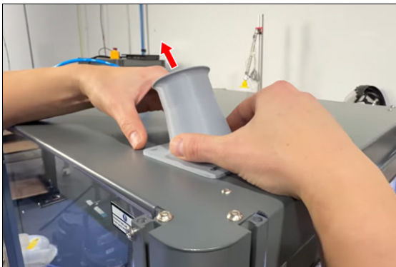
Figure 3-27: Hose guide positioned on the top of the enclosure.
