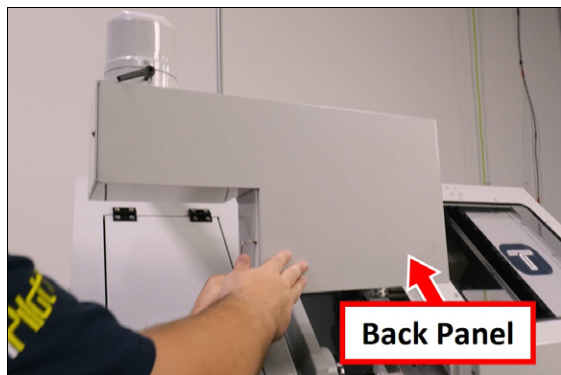
Figure 5-16: Operator console mount's back panel.
