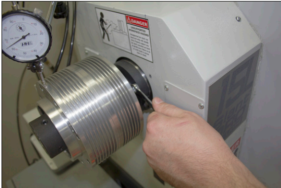
Figure 5-62: Tighten the mounting flange on the pneumatic cylinder.
