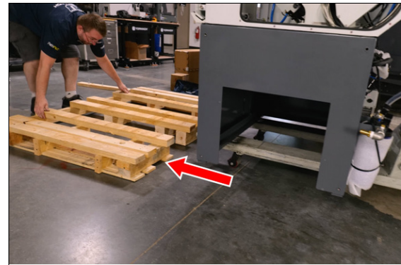
Figure 5-10: Removing the pallet from under the machine.
