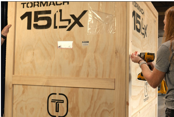
Figure 5-2: Removing the screws from the side panels of the shipping crate.
