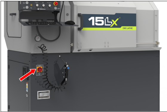
Figure 5-29: The Main Disconnect switch on the side of the machine's electrical cabinet.
