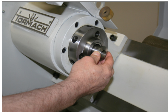
Figure 5-67: Collet installed into the 5C insert.
