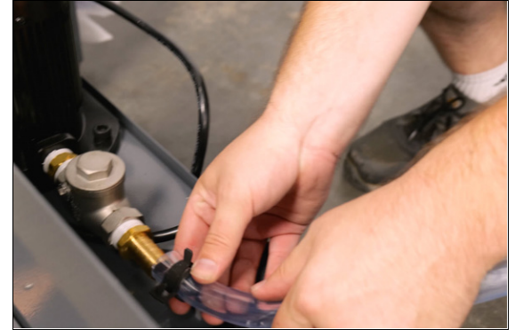
Figure 5-14: Connecting the coolant hose to the coolant pump.
