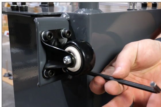
Figure 4-4: Installing the casters onto the coolant tank.
