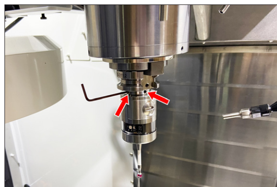
Figure 4-132: Both sets of screws are shown; not shown are each set's opposing screw.
