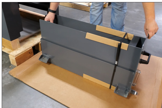
Figure 4-3: Removing the coolant tank from the stand.
