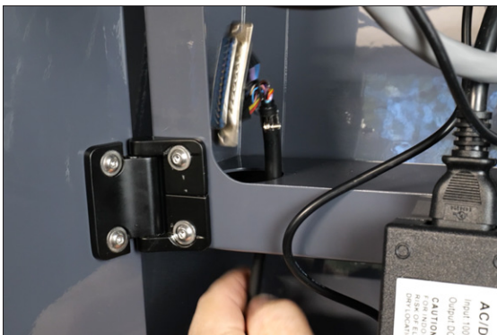
Figure 4-54: Routing the jog pendant cable through the bottom of the operator console mount.
