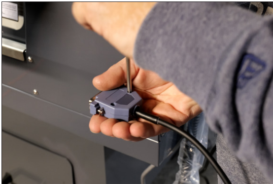
Figure 4-53: Disassembling the jog pendant's DB25 connector.
