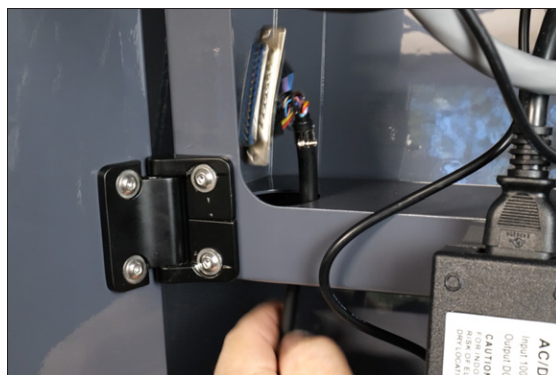
Figure 4-71: Routing the jog pendant cable through the bottom of the operator console mount.
