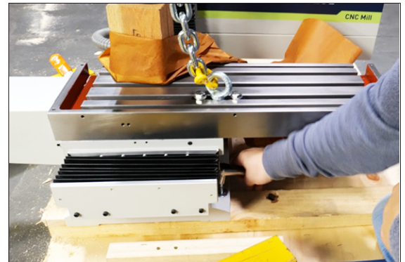
Figure 4-10: Removing the bolts securing the machine to the pallet.
