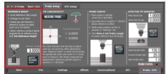
Figure 4-136: Reference height section of the probe setup.
