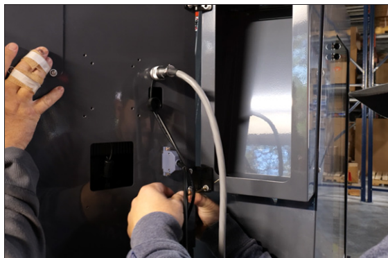
Figure 4-68: Mounting the operator console onto the enclosure.
