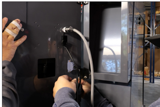
Figure 4-51: Mounting the operator console onto the enclosure.
