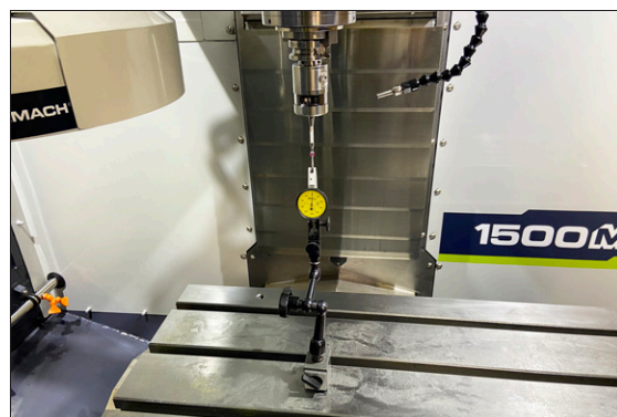
Figure 4-131: Dial indicator set up to check the probe's tip concentricity.
