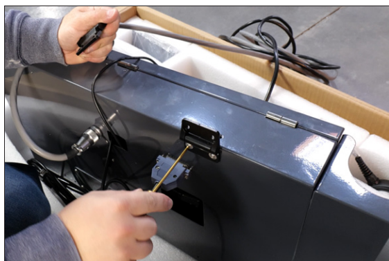
Figure 4-50: Installing the hinges onto the operator console.
