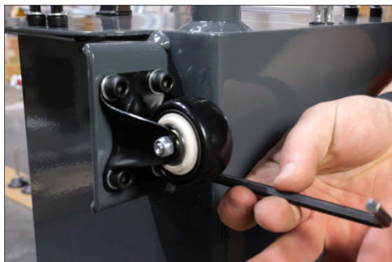
Figure 4-61: Installing the casters onto the coolant tank.
