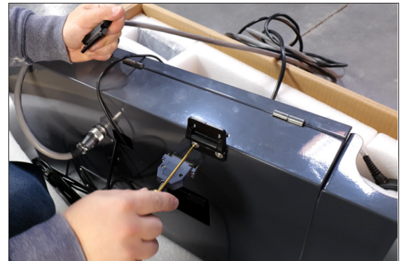
Figure 4-67: Installing the hinges onto the operator console.
