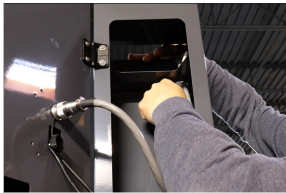
Figure 4-52: Routing the cables through the top operator console mount and to the top of the enclosure.
