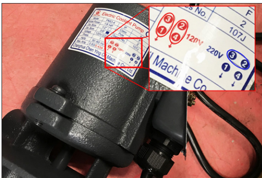
Figure 4-107: Coolant pump motor jumper configuration diagram.
