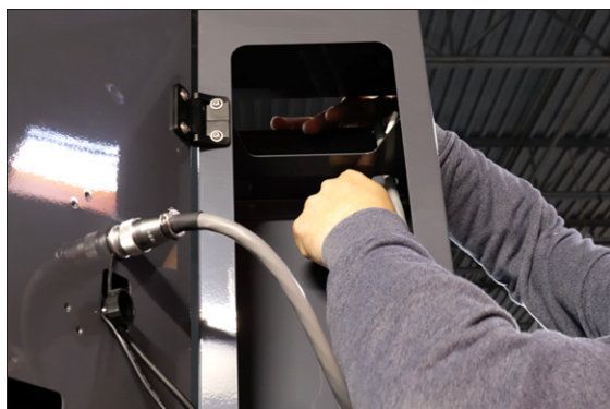
Figure 4-69: Routing the cables through the top operator console mount and to the top of the enclosure.
