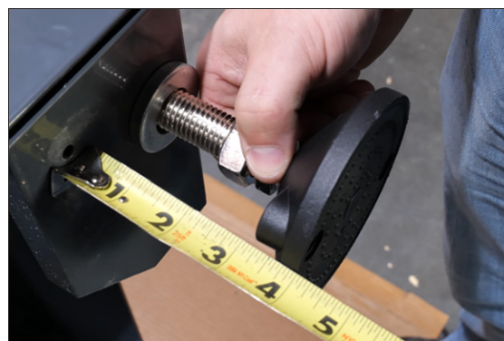
Figure 4-64: Adjusting the height of the foot.
