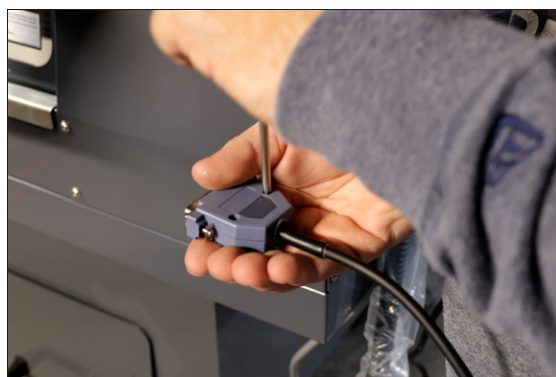
Figure 4-70: Disassembling the jog pendant's DB25 connector.
