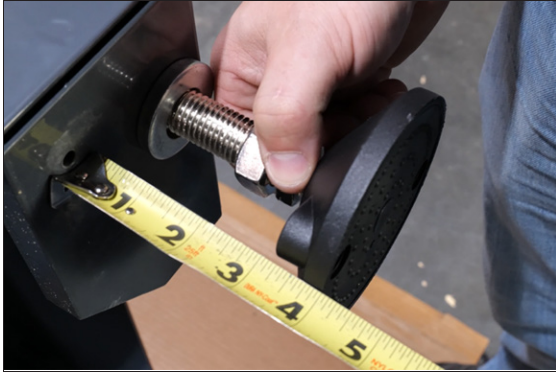
Figure 4-8: Adjusting the height of the foot.
