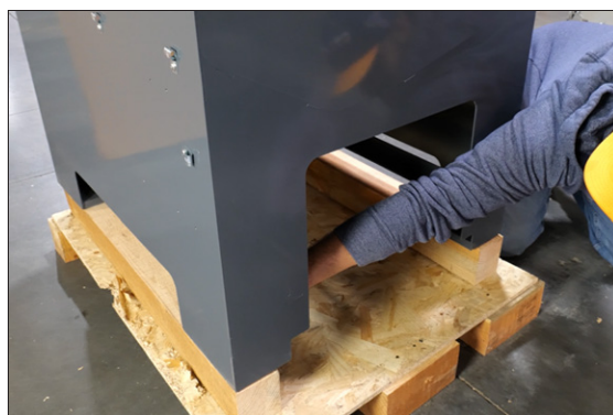
Figure 4-5: Removing the bolts securing the machine stand to the pallet.
