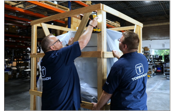
Figure 4-59: Removing the side panels of the shipping crate.
