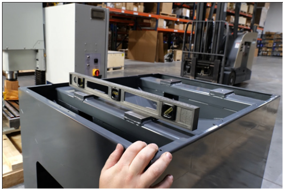
Figure 4-12: Leveling the machine stand.
