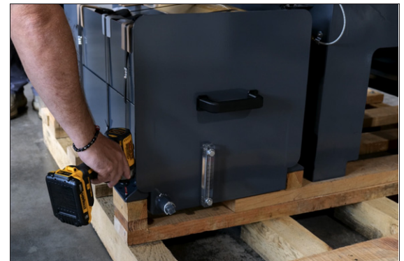
Figure 4-60: Removing the coolant tank's screws from the pallet.
