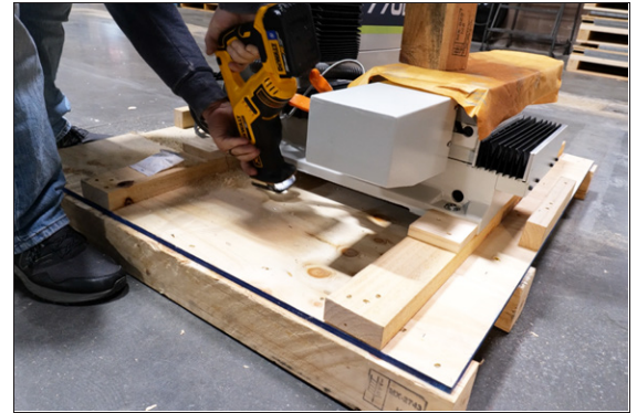
Figure 4-9: Trimming the left side of the machine's pallet.
