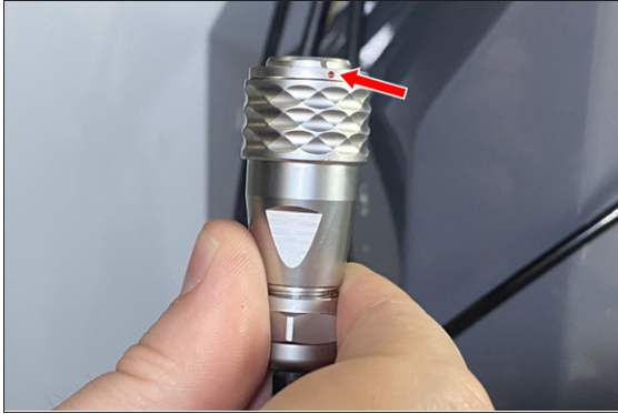
Figure 4-117: Red dot on the cable to align with the red dot on the connector.
