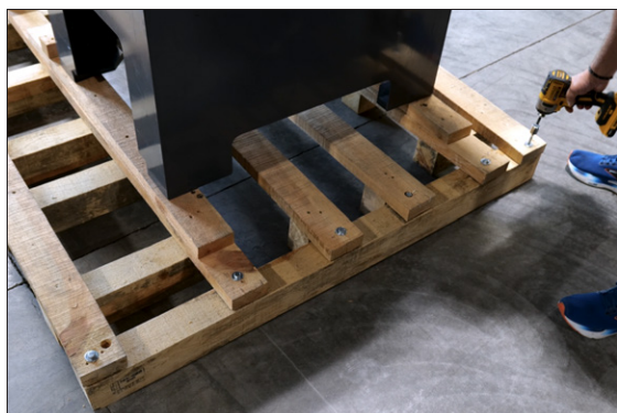
Figure 4-62: Removing the bolts on the right side of the pallet.
