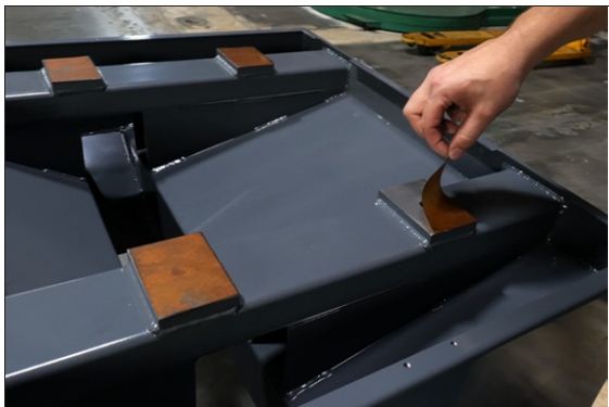
Figure 4-11: Removing the protective stickers from the pads on the machine stand.
