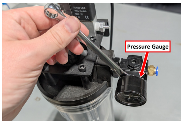
Figure 5: Installing the pressure gauge onto the air pressure regulator.
