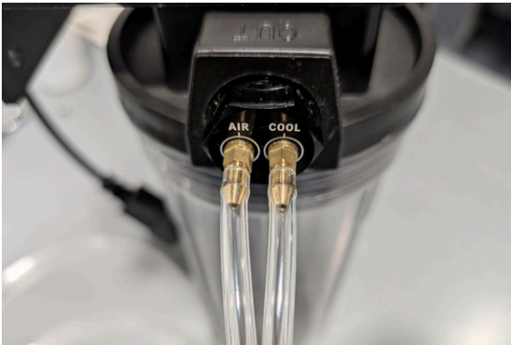
Figure 7: Duplex tubing connected to the canister.
