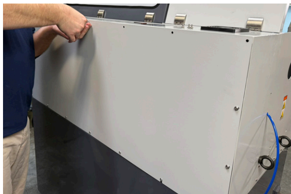
Figure 14: Removing the back panel from the machine.
