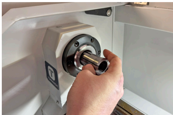
Figure 9: Installing a collet into the spindle.
