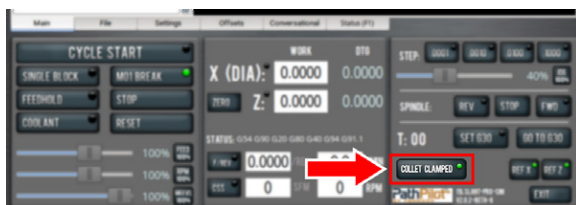
Figure 2: Collet Clamped button with the light on.
