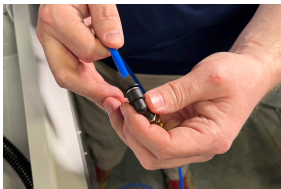
Figure 12: Connecting Hose 3 to the PTC elbow fitting.
