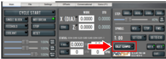
Figure 3: Collet Clamped button's light off.
