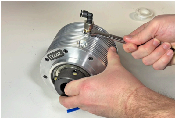
Figure 1: Elbow fittings installed on the pneumatic cylinder.
