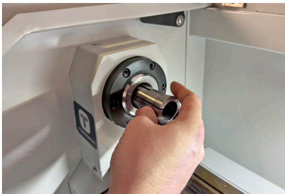
Figure 4: Installing a collet into the spindle.
